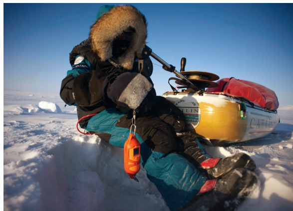
Researchers from the Catlin Survey team deploy a lightweight CTD under Arctic ice to trace effects of melting ice and warmer temperatures.
